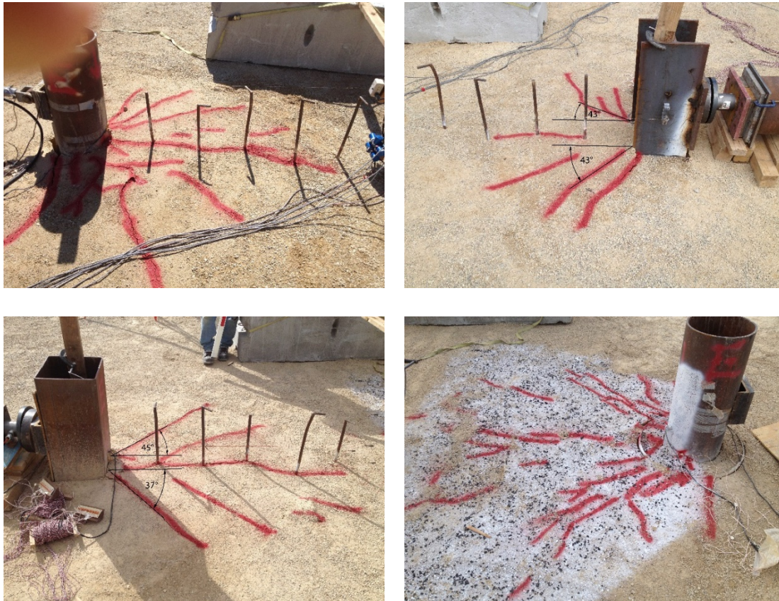
Figure 5-1: Failure Plane around the Piles: Round (top left), H (top right), Square (bottom left), Round in CMS (bottom left)
