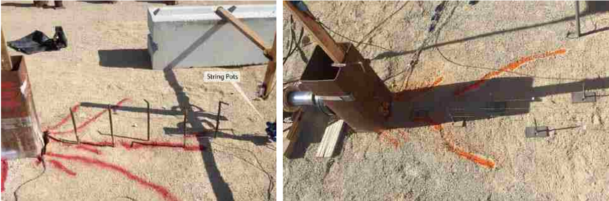
Figure 4-3: String Potentiometers in Place during Testing
