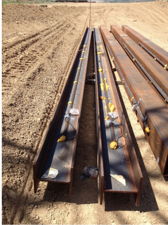
Figure 4-4: Strain Gauges Encased in a Steel Angle
